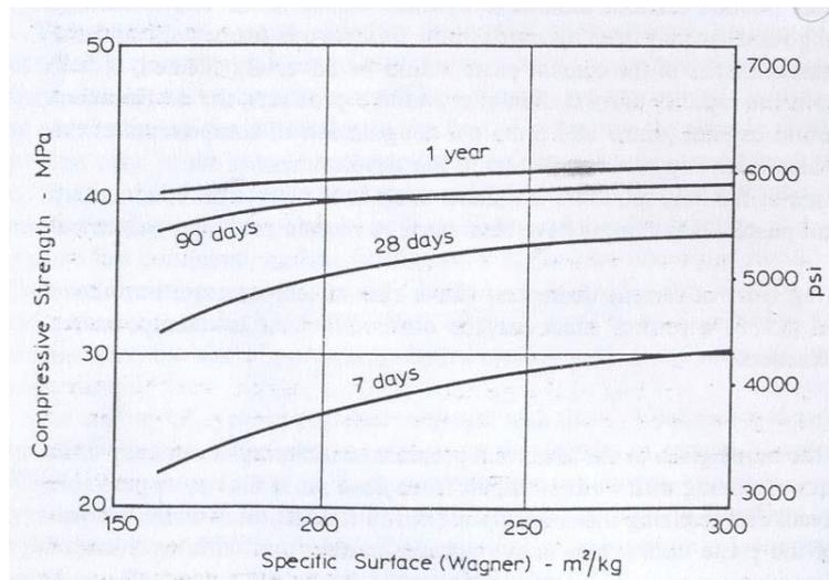
Figure (2): Relation between strength of concrete at different ages and fineness of cement.
