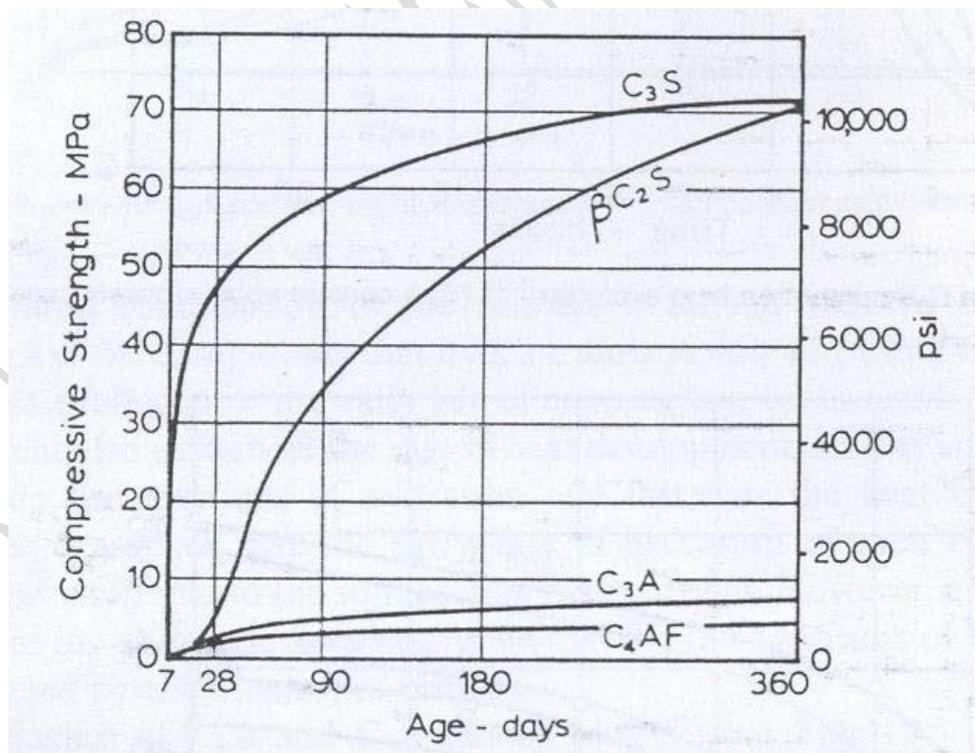
Figure (4): Development of strength of pure compounds according to Bogue.
