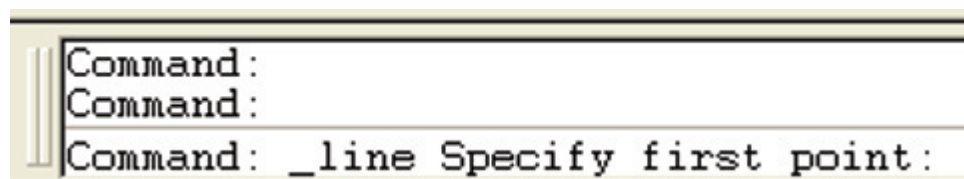
Fig. 2.2 The prompt appearing at the command line in the command palette when Line is "called"
