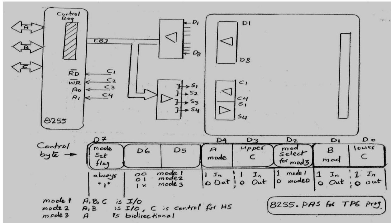
**Fig. 4.3: connection between 8255 and the Centronic experimental board**
