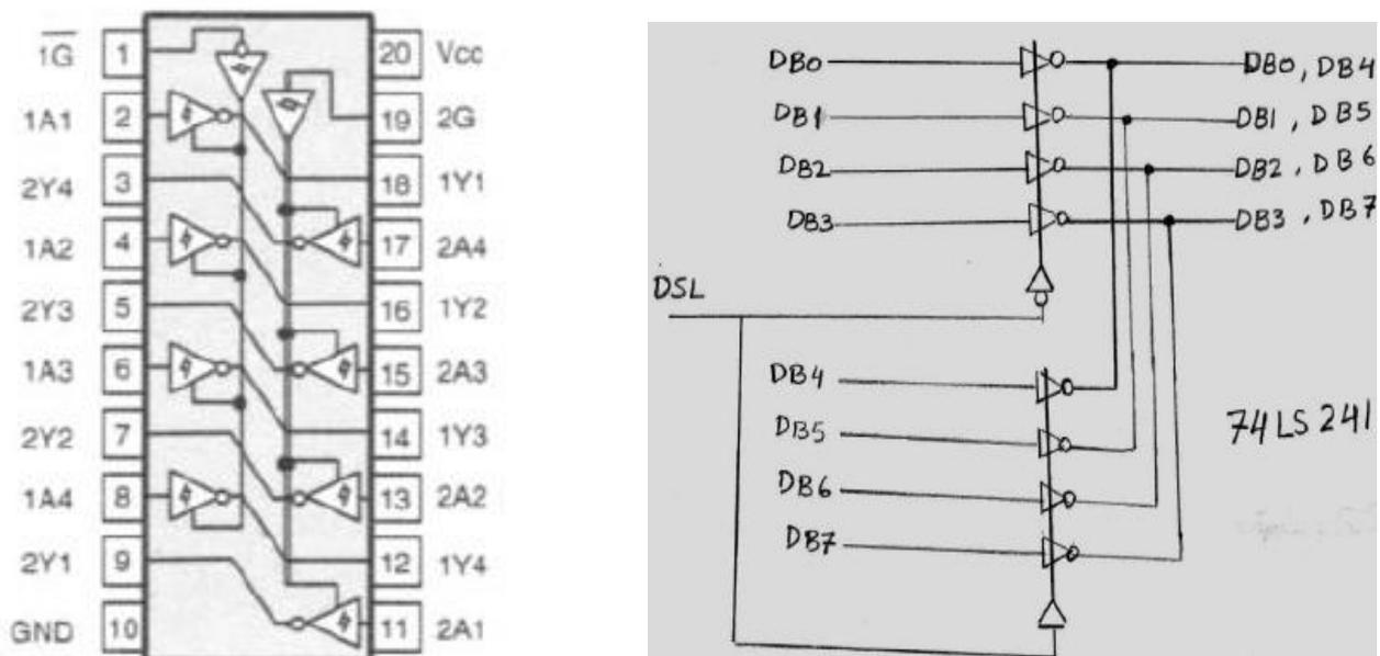
**Fig. 4.1: The pin-out of the 74LS241**
