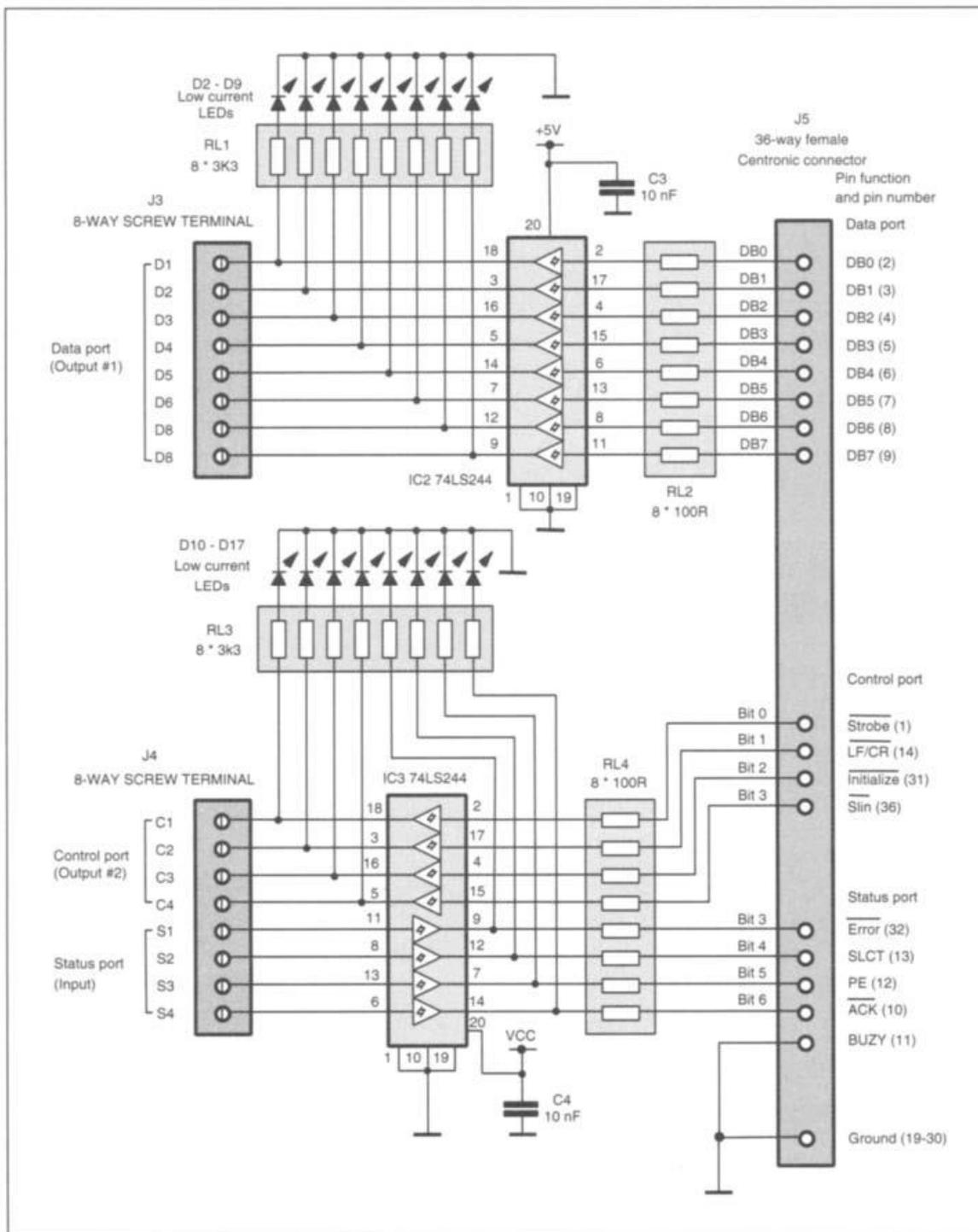
Fig. 2.18: Circuit of the Centronic experimental board
