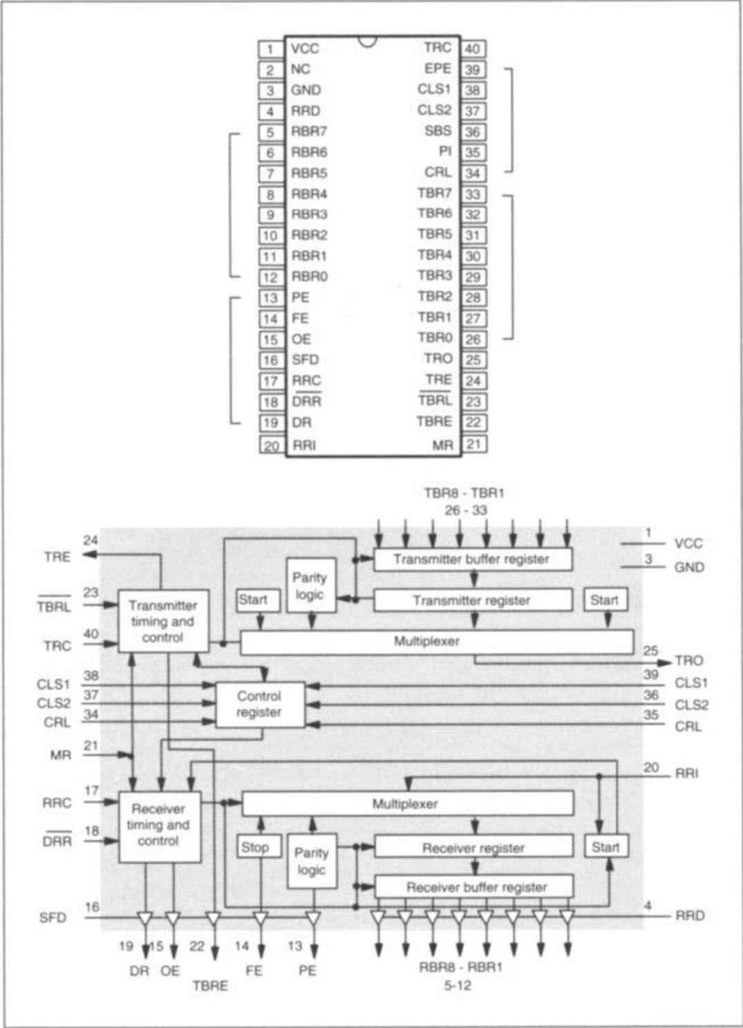
**Figure 4.8 Pin-out and internal block diagram of the 6402 UART**
