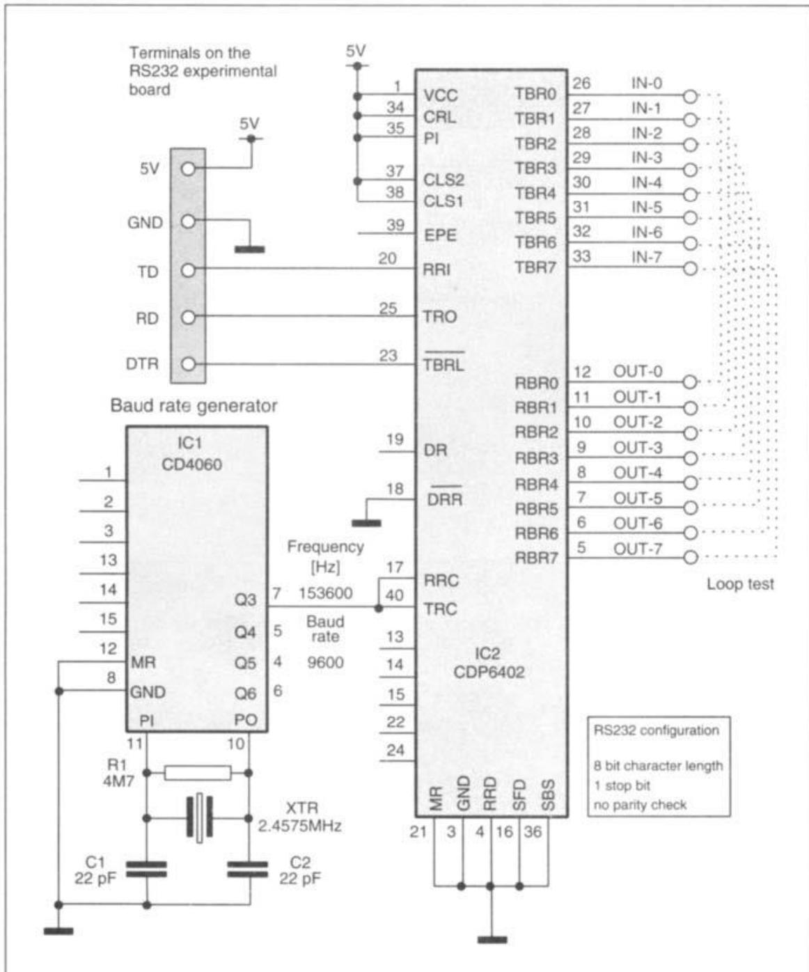
**Figure 4.10 Experimental circuit diagram of the 6402 UART**
