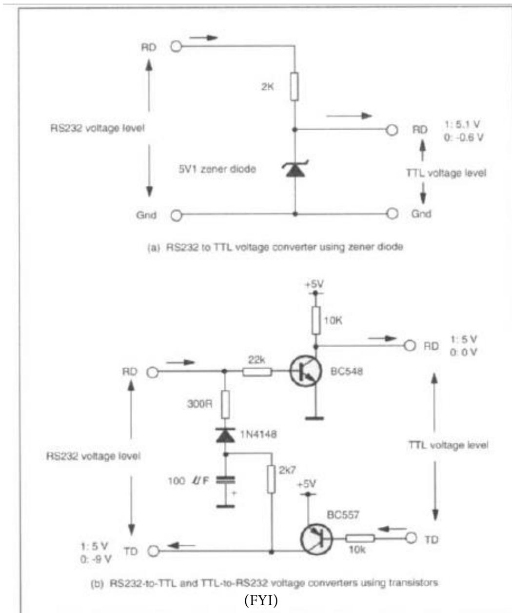
**Figure 4.5 TTL/RS232 voltage converter circuits**
