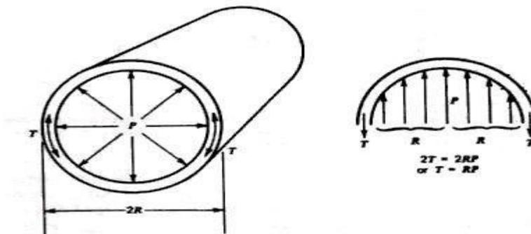
For a long tube of radius  $R$  with blood pressure  $P$  (a) we can calculate the tension in the walls
