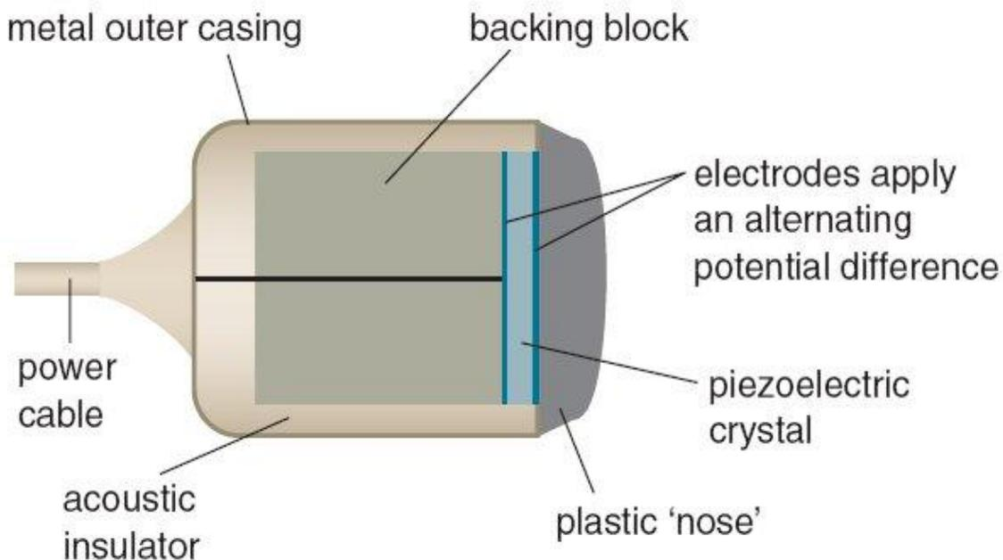
*\* Operation of an ultrasound transducer is based on the piezoelectric effect.*
