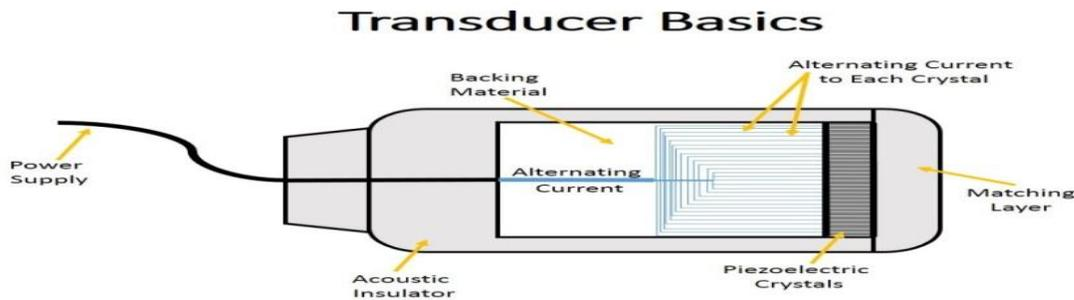
\* The active element of the transducer is *the piezoelectric crystal*. The material most frequently used is *lead zirconate titanate (PZT)*.
