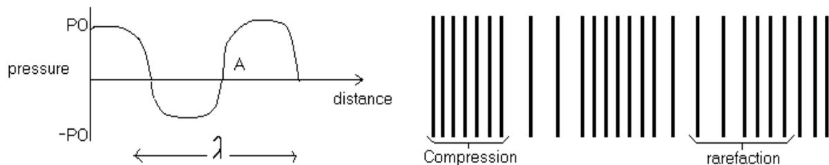
**Figure (1)** A sound wave vibrates at frequency  $f$  and produces compression and rarefaction.
