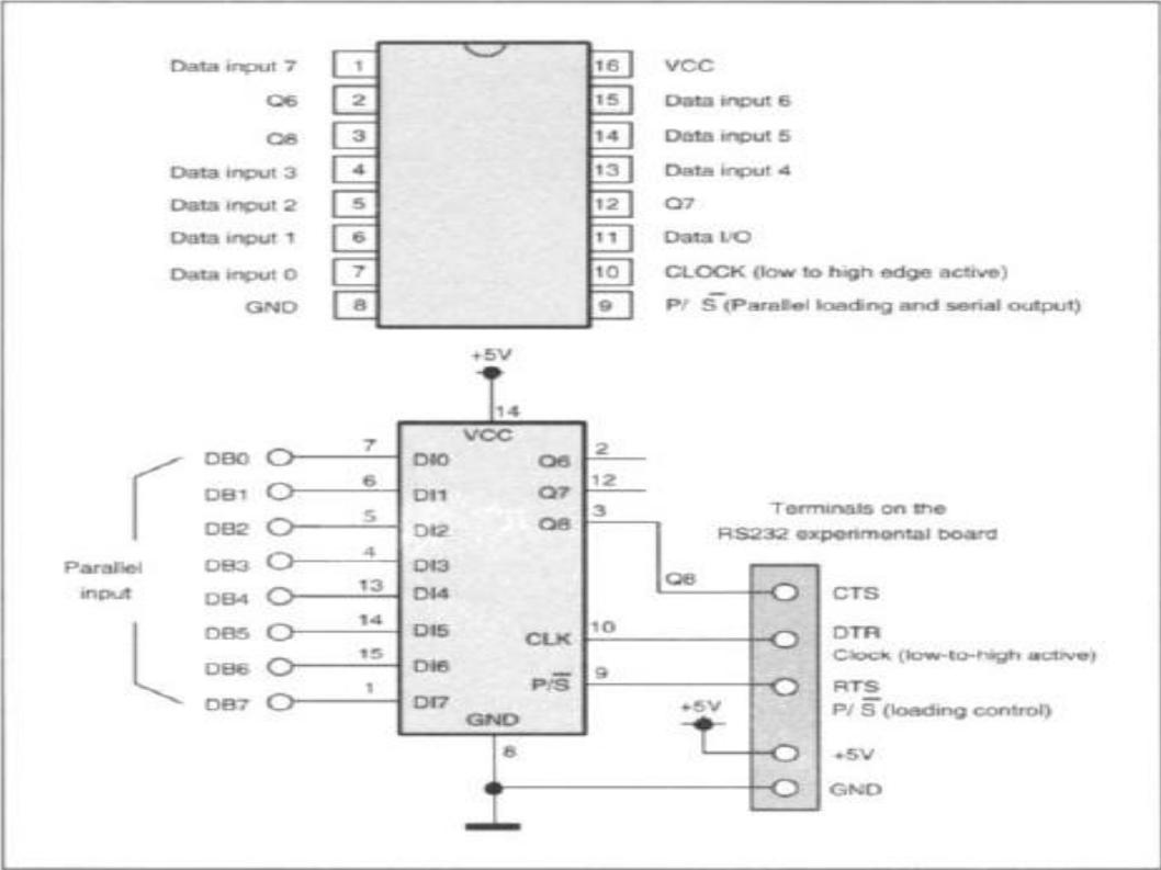
**Figure 4.13 Parallel-to-serial converter using a CD4021 shift register**
