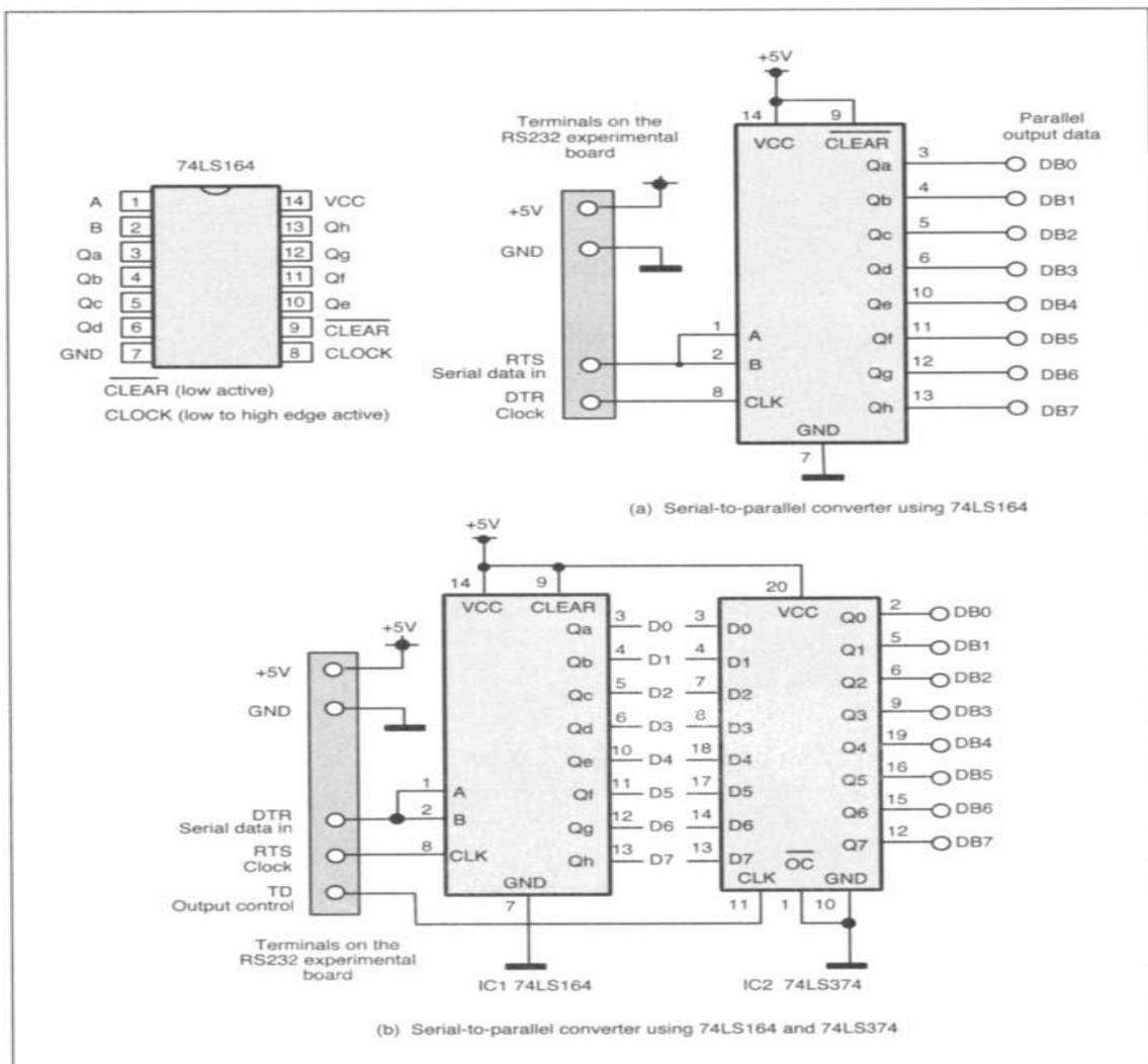
**Figure 4.12: Serial to Parallel convertor circuits using 74LS164 and 74LS374**
