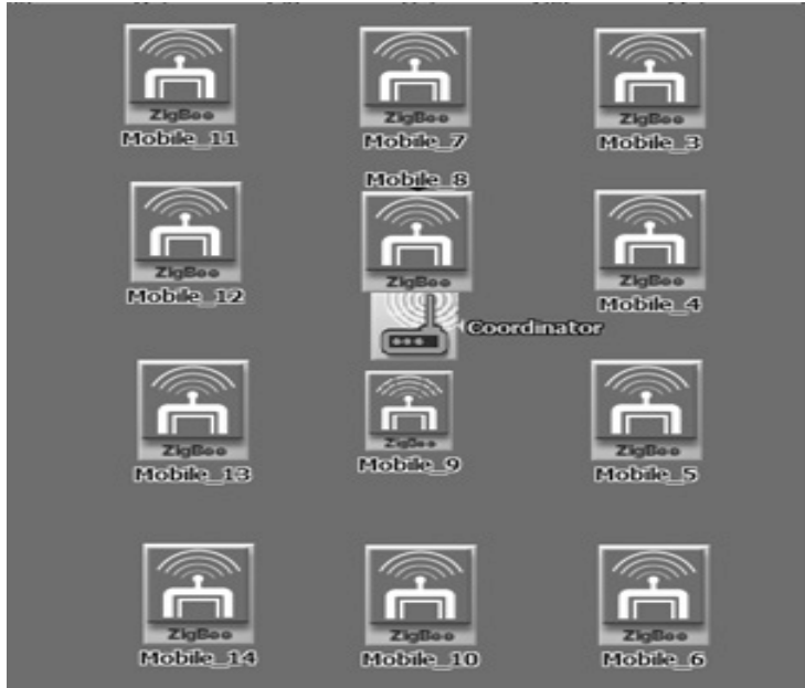
Figure (5) first scenario, 12 Zigbee Nodes with one Coordinator
