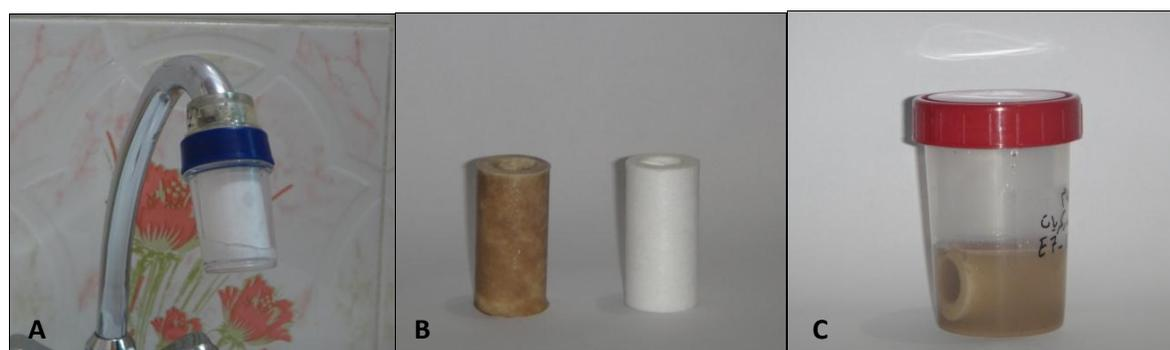
**Figure 1-** A: Domestic filter unit that used in the present study, fixed in a faucet. B: The cartridge filtes, before and after use. C: The cartridge filter immersed in dispersing solution.
