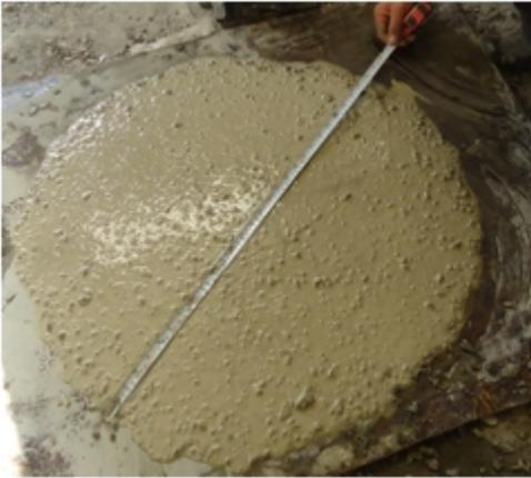
**Fig .(2) Spreading concrete in Slump
